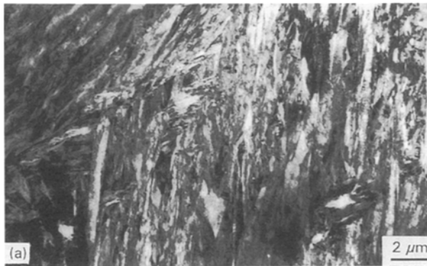
Figure 3 (a) Transmission electron micrograph of the microstructure of sample tempered at 400 °C for 30 min with no applied stress, showing a Widmanstätten array of carbides; (b) as (a), showing regions with only one variant (marked A) and regions with a Widmanstätten array of carbides (marked B).
