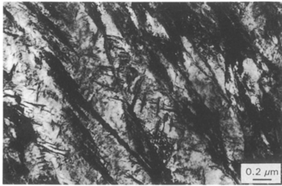
Figure 6 Transmission electron micrograph of specimen tempered at 400 °C for 30 min with an applied compressive stress of 500 MPa, showing some plates containing more than one variant.
