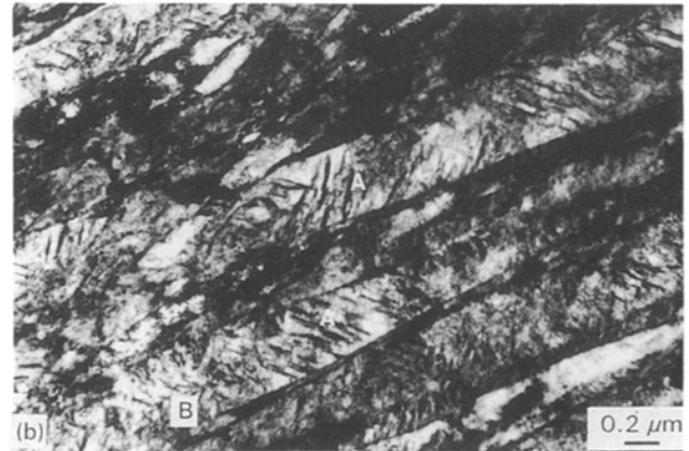
Figure 3 (a) Transmission electron micrograph of the microstructure of sample tempered at 400 °C for 30 min with no applied stress, showing a Widmanstätten array of carbides; (b) as (a), showing regions with only one variant (marked A) and regions with a Widmanstätten array of carbides (marked B).
