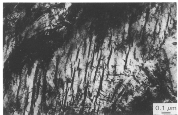
Figure 5 Transmission electron micrograph of specimen tempered at 400 °C for 30 min with an applied compressive stress of 500 MPa, showing a single variant of carbide.
